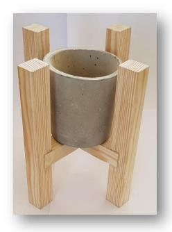
Years 9 and 10 have made plant stands with pots cast from cement using repurposed take-away drinks cups. As an introduction to the GCSE course, this practical work reinforced the theory topics in timbers, joining methods, casting and technical drawing. Casting in concrete gave students the opportunity to work with a material they may not have used before and allowed them to problem solve and experiment with different moulds.
