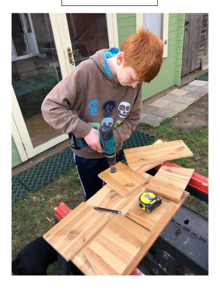
I am using a drill with a circular hole cutter. I am making the hole for the birds to go in.
